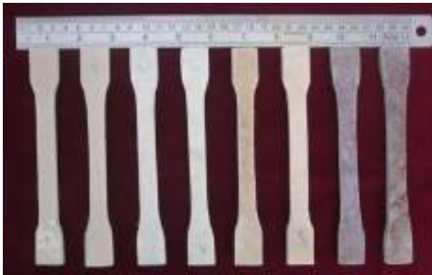
Fig. 3: Tensile specimens (before testing)
