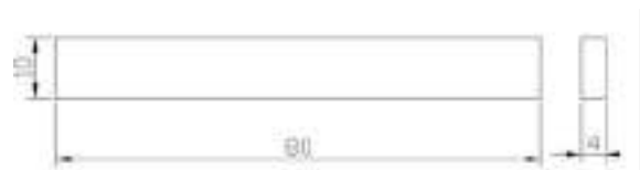
Fig.8: ASTM D 790 standard flexural specimen
